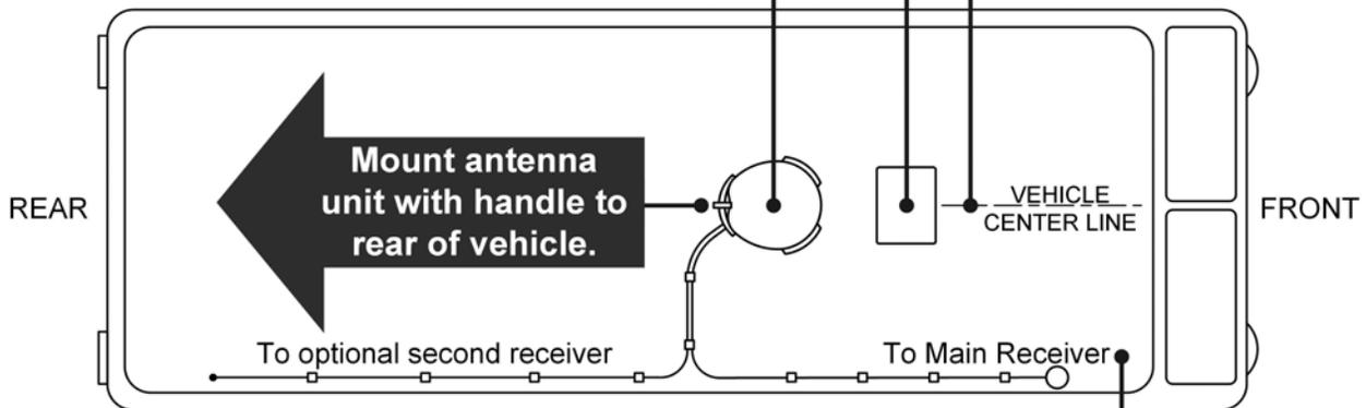
**Try to install antenna unit as close as possible to main receiver to minimize coax length.**
