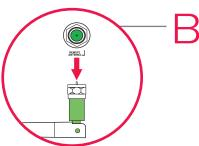
Locate the antenna connected to the "Remote Antenna" port. Then unscrew the antenna from the receiver.
