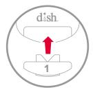
**3** Move the signal switch on the back of the remote from *UHF* to *IR* using the tip of a pen
