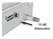
3 Attach the remote control antenna to the newly installed attenuator.
