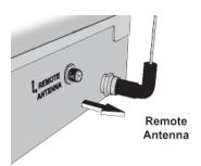
2 Attach a 10 dB attenuator directly to the **REMOTE**ANTENNA input.
